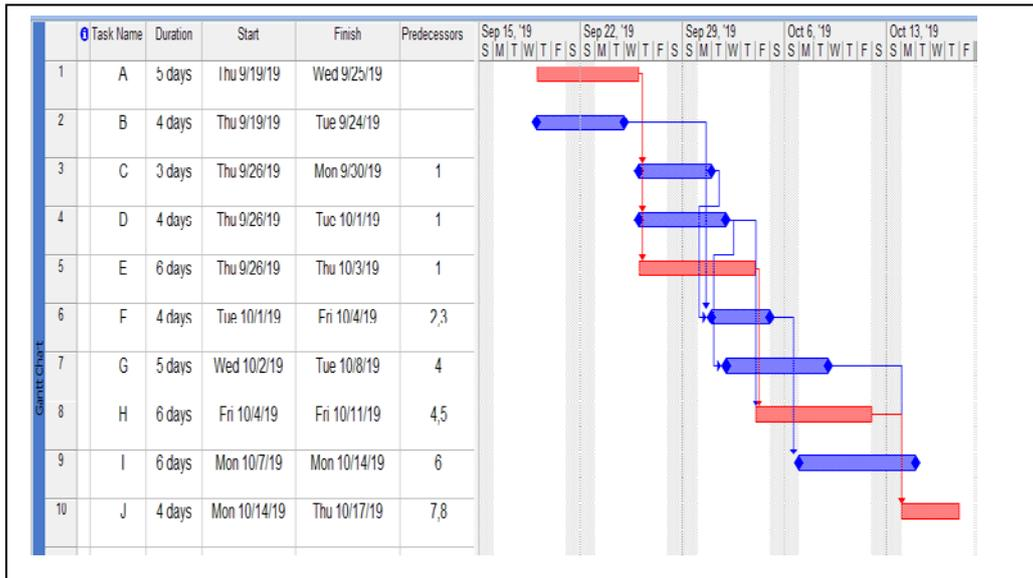
Figure 9 A Gantt chart of a sample project from Table 2 data in MS Project
